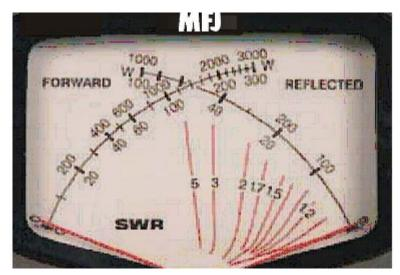
This is a typical meter that you would use to measure an antenna system. With it you can measure swr as well. This type of meter will only show you the swr at the frequency that you are currently on. How do you make an swr chart from this?
